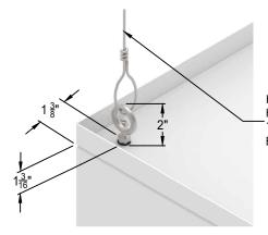
EACH ULTRASUITE MODULE COMES WITH 4 EYE BOLTS FOR HANGING. PRICE RECOMMENDS HANGING EACH UNIT INDIVIDUALLY WITH THE FOUR RECOMMENDED MOUNTING POINTS PER MODULE
